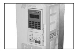
FIGURE 12: VFD key pad & LCD
